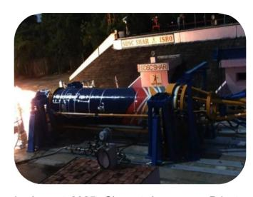
In August 2025, Skyroot Aerospace Private Limited (SAPL) achieved a significant milestone by successfully conducting the first static test of the KALAM-1200 solid rocket motor. This motor serves as the first stage booster of the Vikram-1 Launch Vehicle (LV). The test took place at the Satish Dhawan Space Centre (SDSC) located in Sriharikota, Andhra Pradesh, marking a key advancement in the development of India's private sector-led space capabilities.
